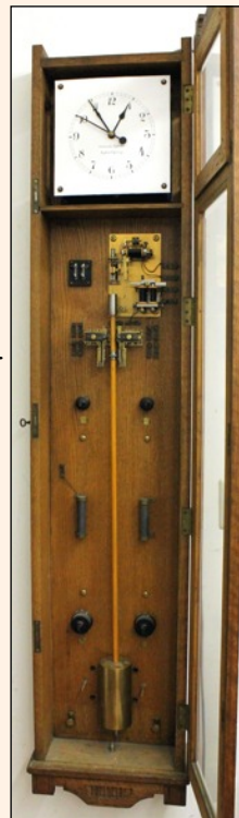
Above: Two views of the seconds type slave dial movement.
