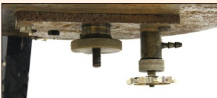
Above: A view below the clock which shows the vacuum valve and the knob which raises and lowers the pendulum in order to lock it during transportation. It operates within a steel bellows inside the clock so as to maintain the integrity of the vacuum. It's a rather clever setup.
