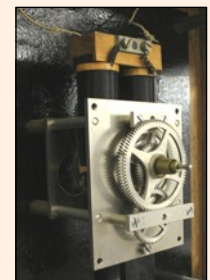
Above: Two views of the seconds type slave dial movement.
