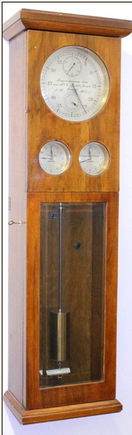
The slave clock used in conjunction with the free pendulum contained in the vacuum tank. It contains the unique pendulum synchronizer.
