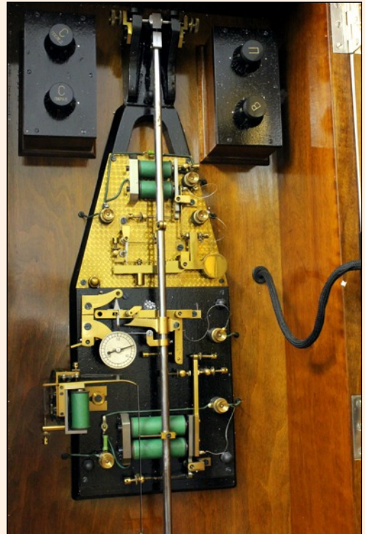
Above: Details of the slave synchronizing movement Below: Pendulum, beat plate and voltage meter
