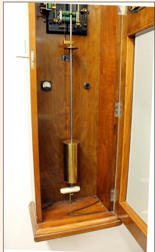
Above: Details of the slave synchronizing movement Below: Pendulum, beat plate and voltage meter
