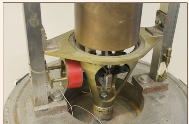
Below: Showing the bob in the unlocked position. You can see at the bottom of the clock, the steel bellows which is shown compressed. It is used to enclose the bob locking mechanism in order to maintain the vacuum in the bell jar. Chamber. It expands when locking ring is raised to lock the bob.
